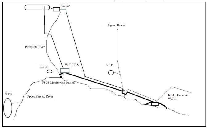
Figure 1. Location of key water supply infrastructure at the confluence of the Pompton and Passaic Rivers. NJDWSC treatment plant (W.T.P) is shown at the top of the illustration. NJDWSC pump station (W.T.P.P.S.) is adjacent to the USGS station. Locations of the sewer treatment plant discharge locations (S.T.P.) are shown as well
