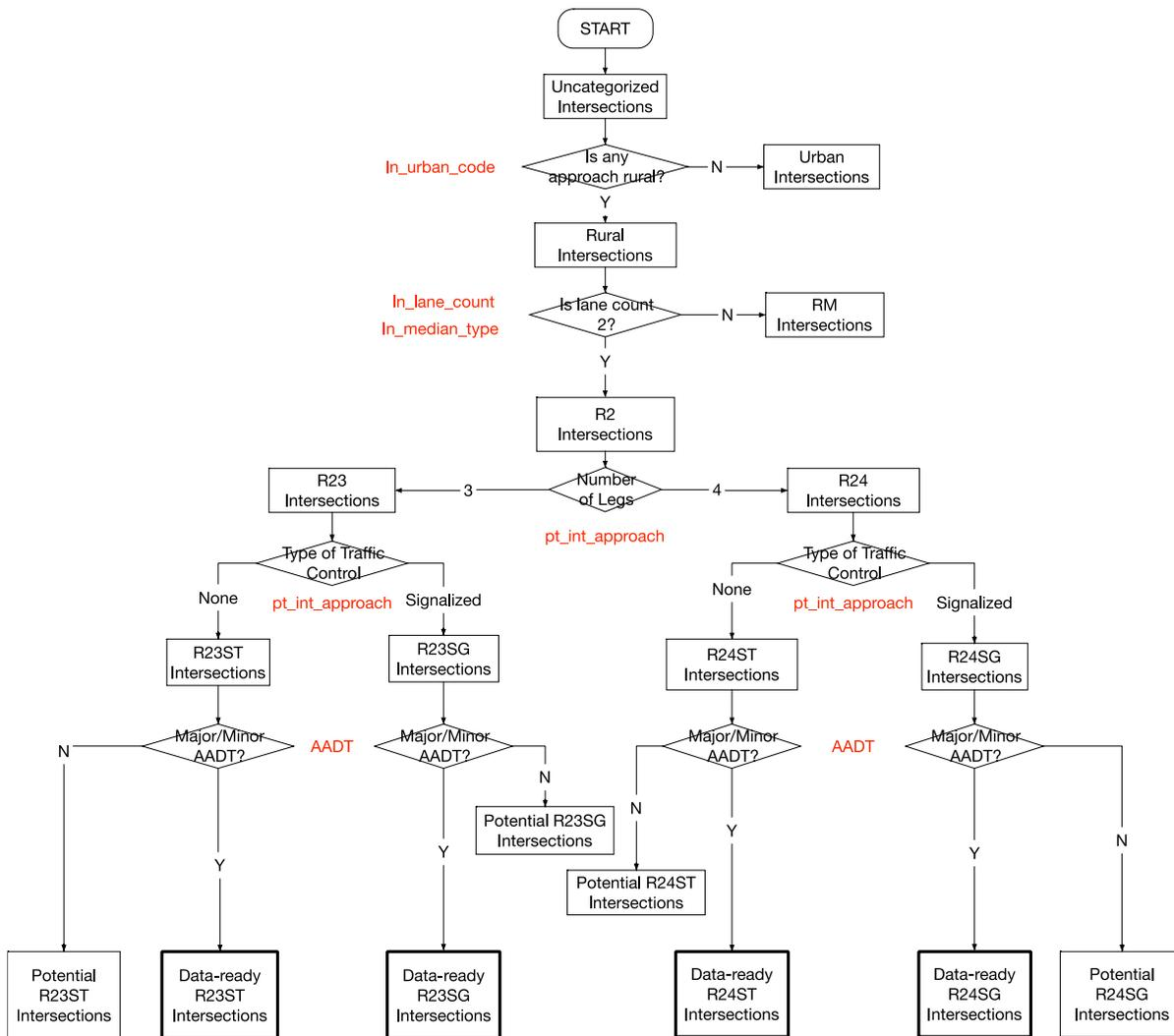
**Figure 19:** Flowchart for identifying the type of data-ready R2 intersections
