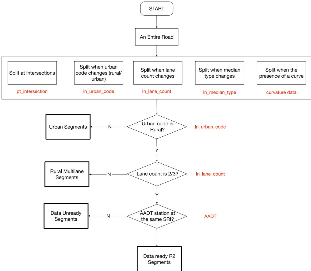
**Figure 15:** Flowchart for automatic detection of R2U
