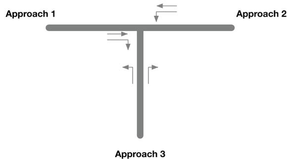
**Figure 46:** An example of a three-leg intersection
