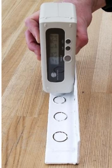
Figure 12. Konica Minolta CR-10 Plus Color Reader
