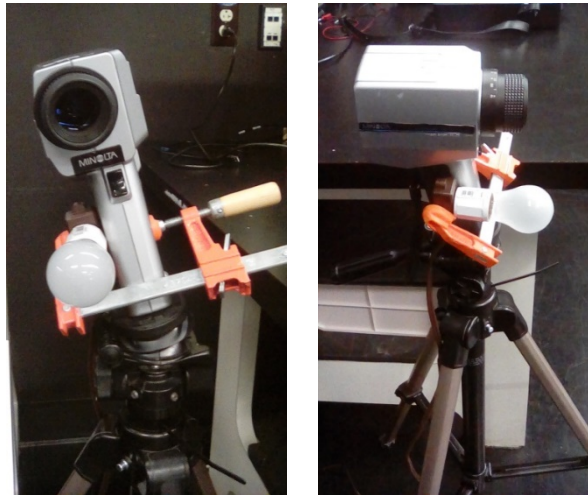
Figure 27. Luminance meter and light source (left: front view, right: side view)
