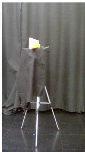
Figure 29. Yellow delineator sample mounted on tripod
