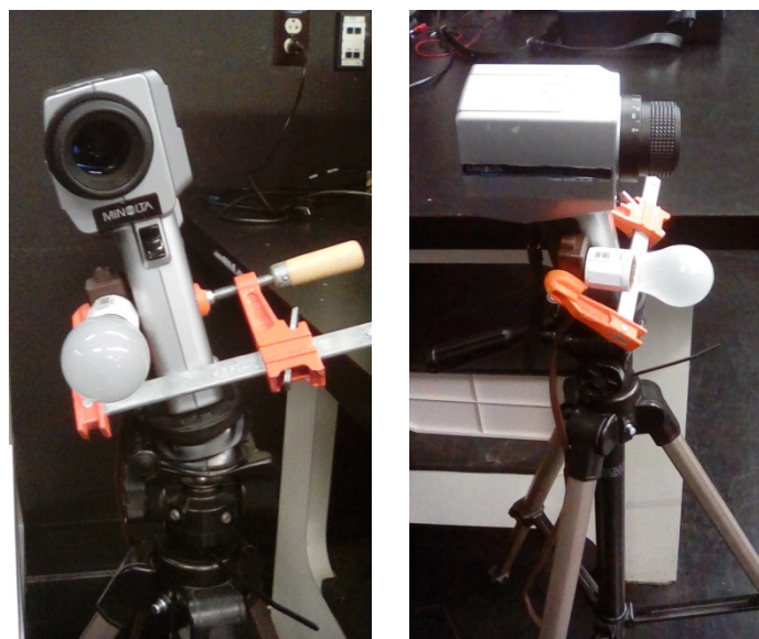
Figure 18. Luminance meter and light source Left: front view. Right: side view
