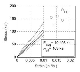
c) Carbon composite tension test results
