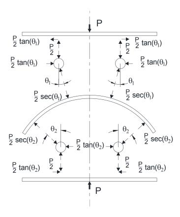
Figure 19. Free-body diagram of arch with roller supports
