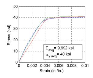
a) Steel tension test results
