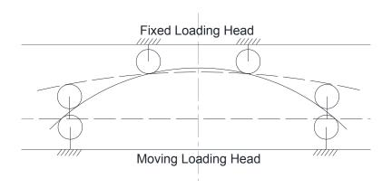
Figure 18. Arch in testing machine supported over rollers
