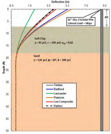
Figure 4: Pile and soil information
