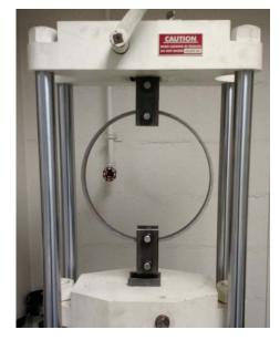
b) Ring fixture in universal testing machine
