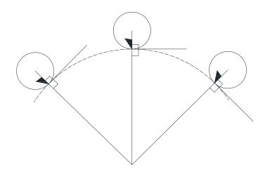
Figure 20. Geometric relationship between rollers and arch
