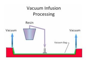
Figure 5. Vacuum Infusion (Moldefiberglass, 2016)
