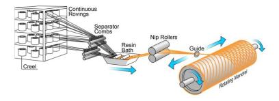
Figure 4. Filament winding process(Nuplex, 2016)
