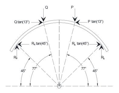
Figure 22. Initial structural anlysis model.
