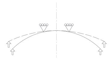
Figure 16. Arch mechanism with two roller supports
