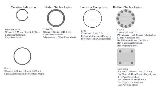
Figure 2. Polymer pile materials
