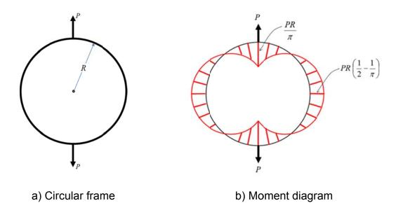
Figure 10. Structural models of the ring test
