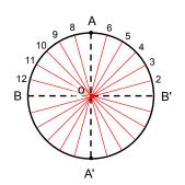
d) Generate 12 diameters at 15° increments
