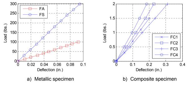
Figure 8. Load-deflection beahior of flexural coupons
