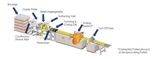
Figure 3. Pultrusion process (Creative Pultrusion, 2016)
