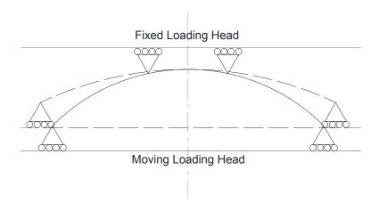
Figure 17. Arch in testing machine
