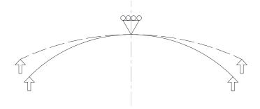
Figure 15. Arch mechanism
