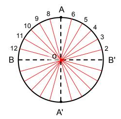
d) Generate 12 diameters at 15° increments
