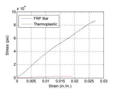
Figure 30. Stress-strain comparison for FRP reinforcing bar and thermoplastic
