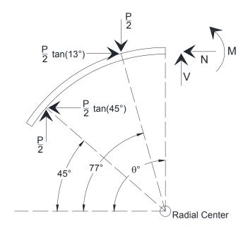
Figure 21. Arch internal force system
