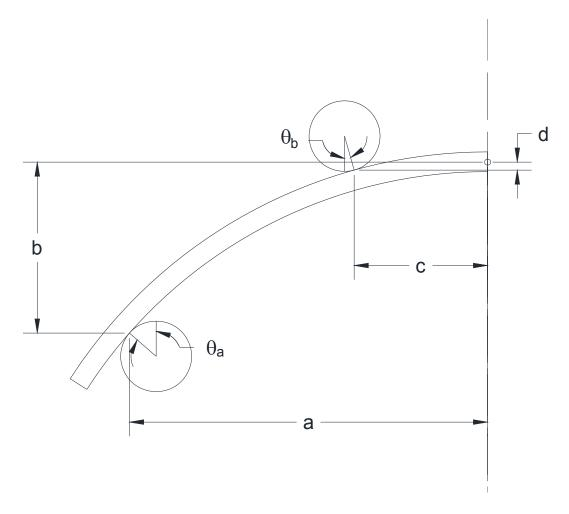
Figure 29. Geometry of deformed arches
