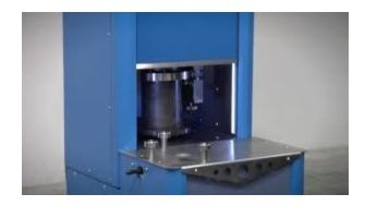
4. ITS breaking head for 6 inch diameter specimens
