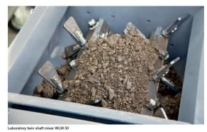
Note: Inspect the sample after mixing to ensure that the mixed material is not packed against the sides of the mixer. If this situation occurs, mix a new sample at a lower moisture content. Check to see that the material mixes easily and remains in a "fluffy" state. If any dust is observed at the end of the mixing process, add small amounts of water and remix until a "fluffy" state is achieved with no dust.
