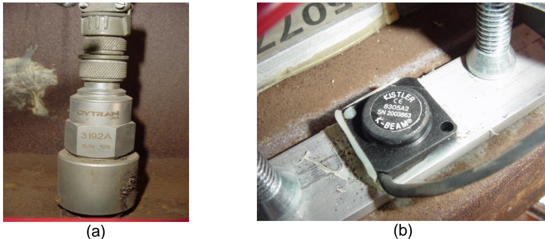
Figure 10. Accelerometers: (a) uniaxial Dytran (model 3192A) and (b) low-frequency Kistler (models 8330A2.5 and 8305A)
