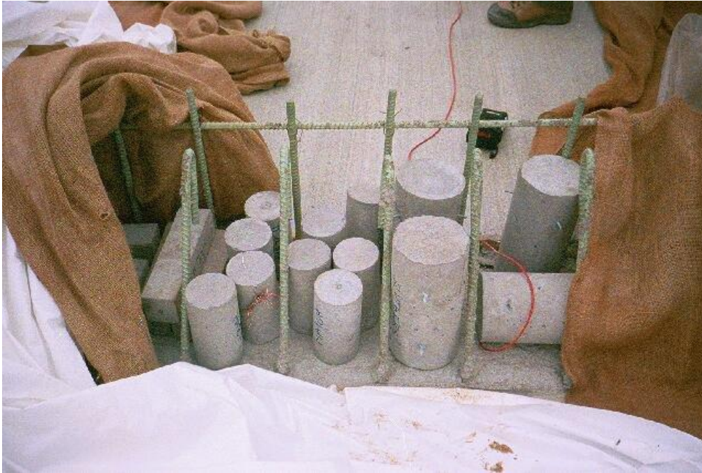
Figure 14. Field matched-cured specimen
