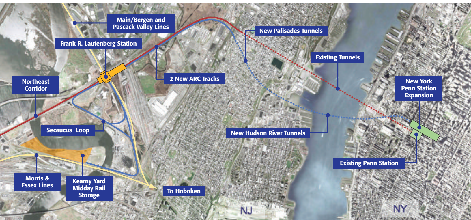
The "Access to the Region's Core" project will include a new commuter rail tunnel under the Hudson River that will connect to a new rail station at 34th Street in Manhattan.
