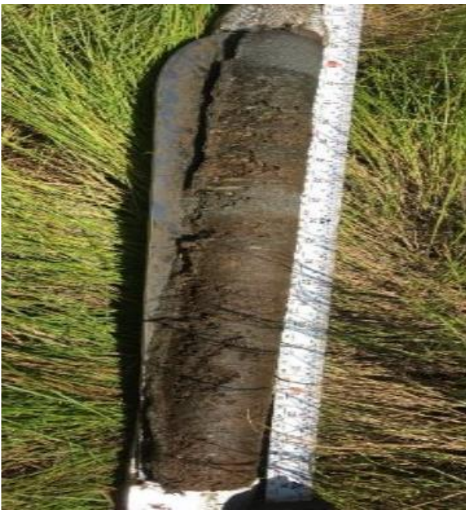
Figure 4. a) Eijkelkamp Peat-coring system ( https://en.eijkelkamp.com/products/augering-soil-sampling-equipment/peat-sampler.html ); and b) sediment core increment obtained at the Cheesequake State Park site.
