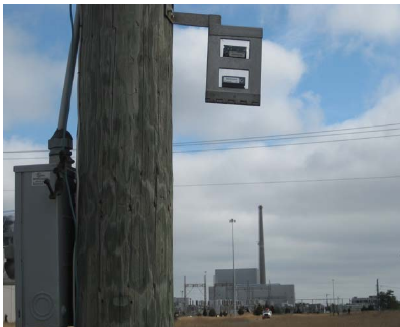
Figure 3 – TLD Used in the Environment
