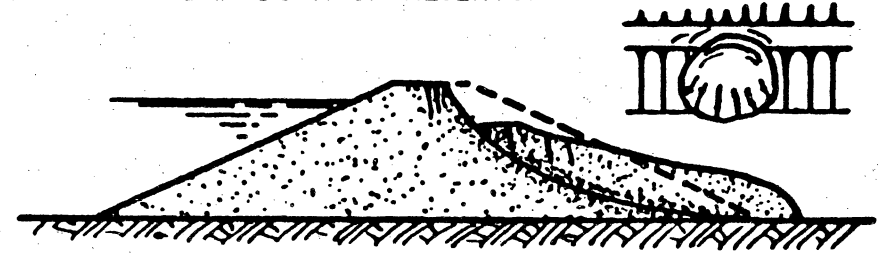
(g) DOWNSTREAM SLIDE DUE TO WEAK EMBANKMENT
