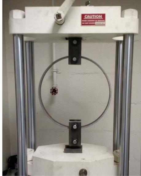
b) Ring fixture in universal testing machine
