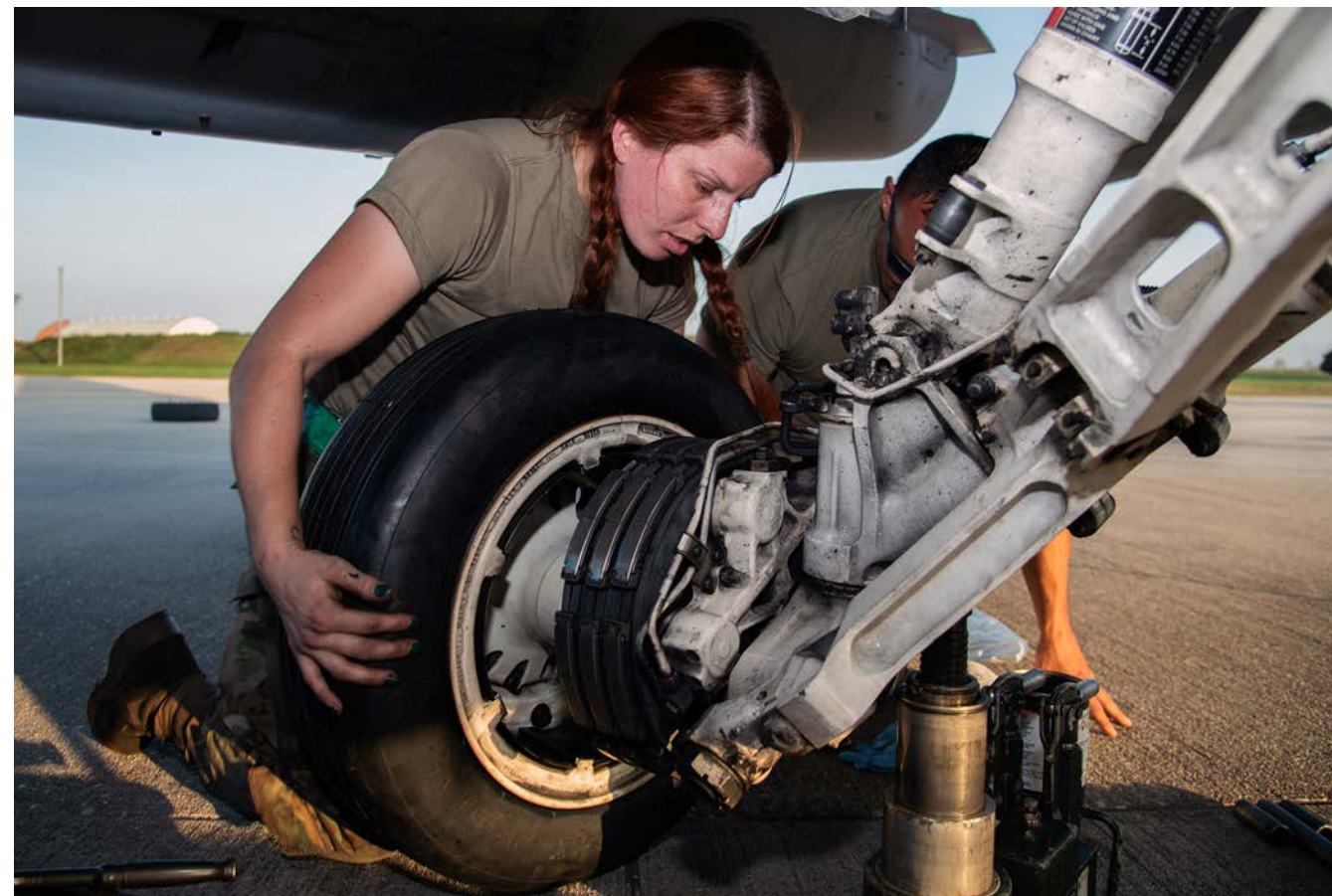
Above: U.S. Air Force Tech. Sgt. Sabrina Hyde, tactical aircraft maintainer, 177th Maintenance Squadron, instructs Tech. Sgt. Rocco Lazaro on how to replace a tire on an F-16C Fighting Falcon with the 177th Fighter Wing, New Jersey Air National Guard, at Aviano Air Base, Italy, Oct. 21, 2024.
