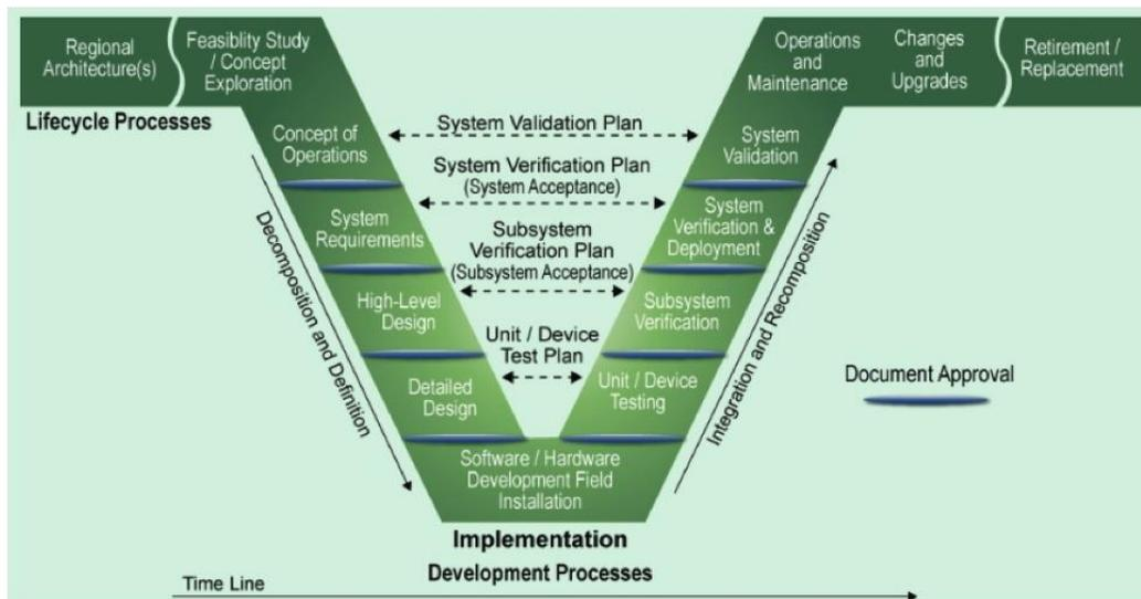
Figure 76. FHWA Systems Engineering “V” Model
