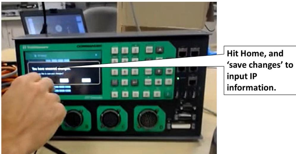
Figure 96. Trafficware Commander Initializing Controller- Saving IP data
