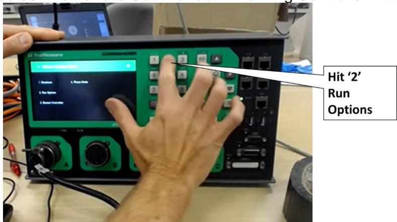
Figure 91. Trafficware Commander Initializing Controller-Run Options
