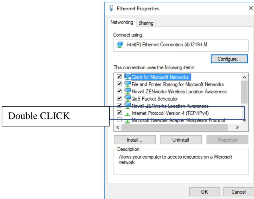
Figure 102. Select Properties for Internet Protocol Version 4 (TCP/IPv4)
