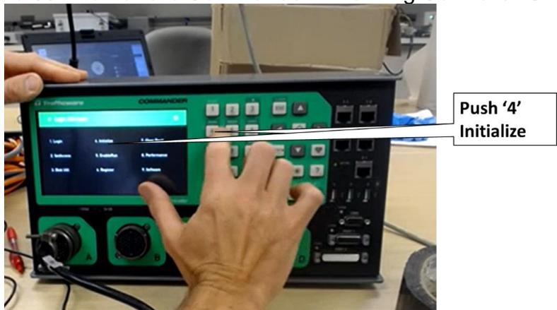
Figure 90. Trafficware Commander Initializing Controller-Initialize
