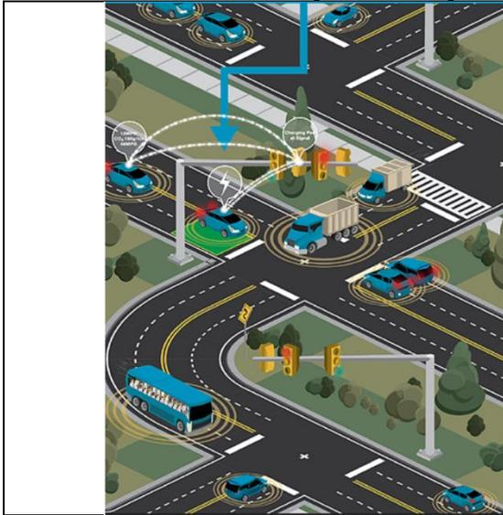
Eco-Traffic Signal Timing is a V2I application to decrease fuel consumption and decrease air pollutant emissions on arterials by optimizing the performance of traffic signals. Vehicle location, speed, and emissions data will be collected to develop adaptive signal timing strategies to reduce idling stops, unnecessary accelerations, and decelerations and improve traffic flow in real-time at intersections, along a corridor, or for a region.
