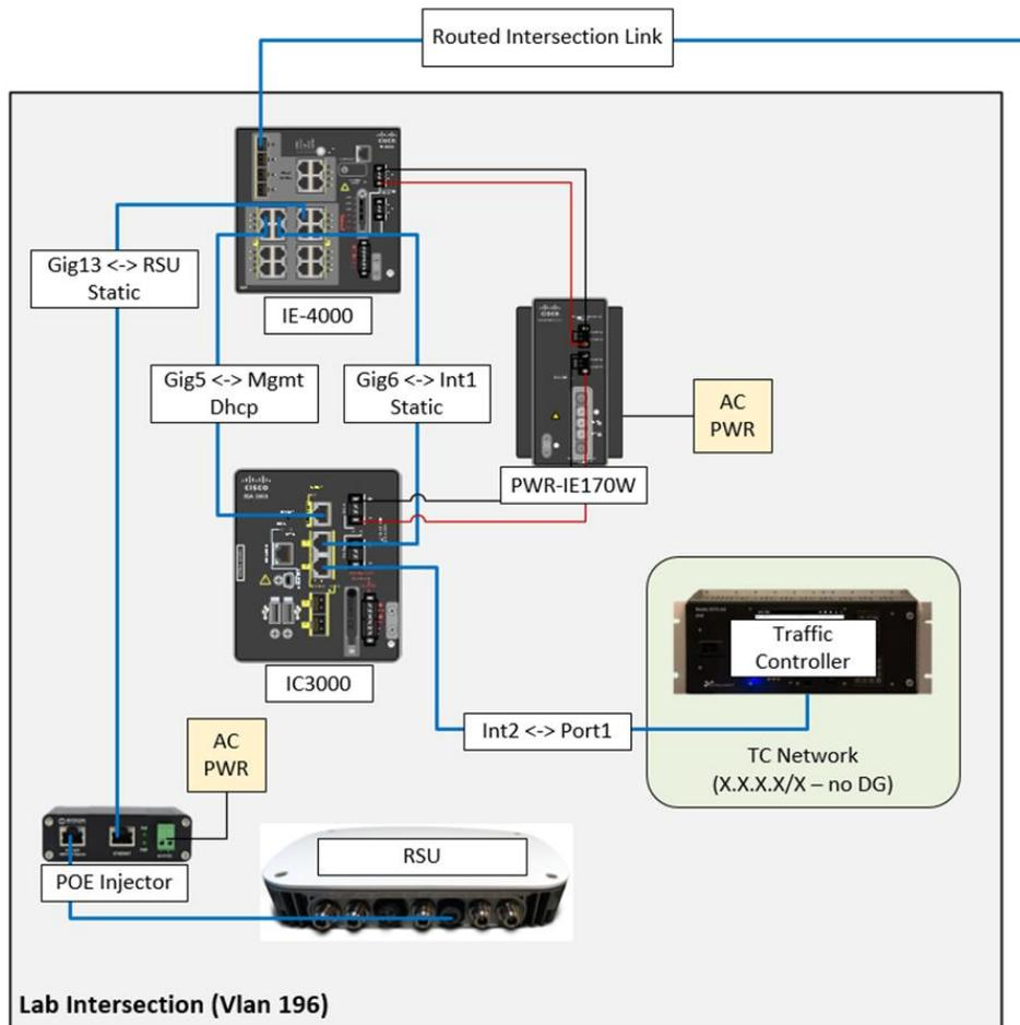
Figure 79. Intersection Level Design
