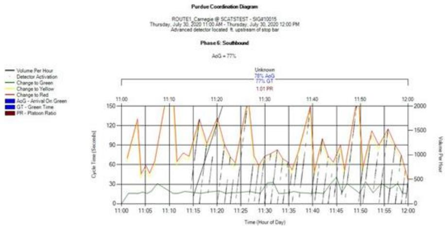
Figure 60. Actual Wavetronix data overlaid on PCD indicating a vector speed (1 hour) for southbound lane 2 at Carnegie and US 1
