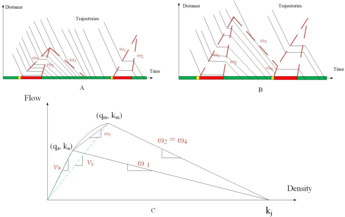
Figure 32. Shockwave and Fundamental Diagram (A. Under-Saturated Condition; B. Over-Queuing shockwave:
