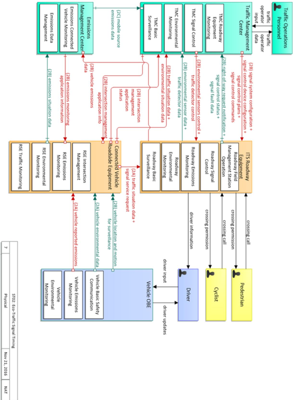
Figure 7. The architecture of Eco-Traffic Signal Timing
