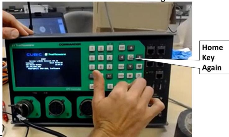
Figure 87. Trafficware Commander Initializing Controller 'Home Key' again if needed.
