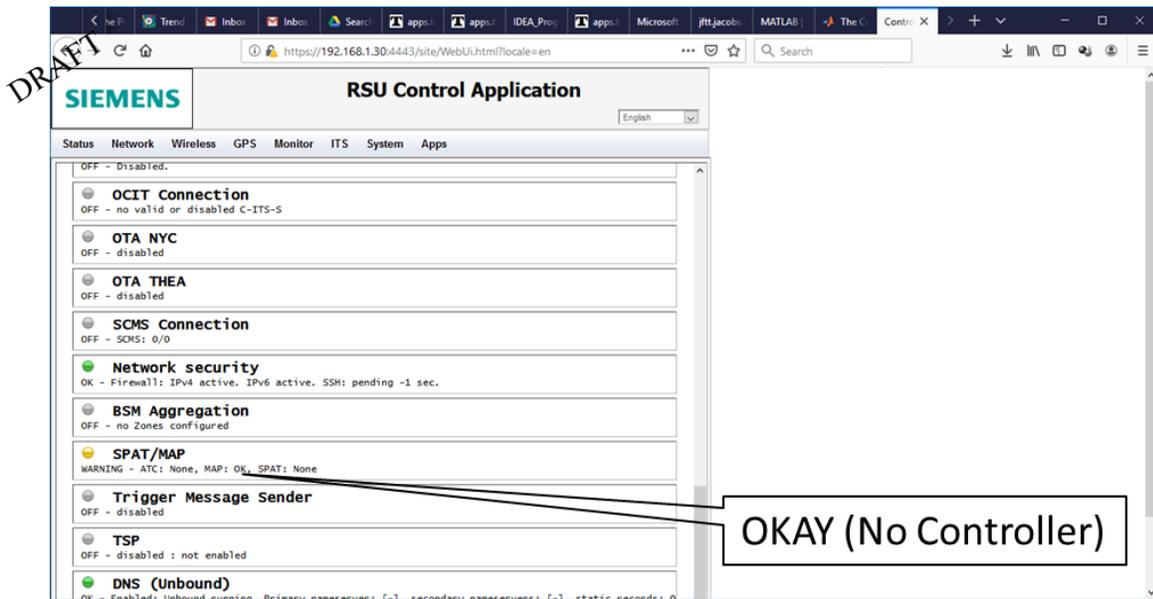
Figure 114. RSU setup, but no controller set with MAP message
