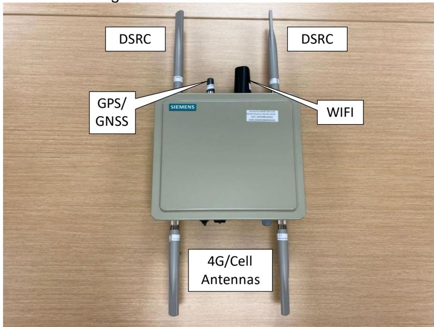
Figure 107. Assembled RSU
