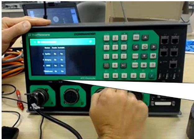
This is a touch screen, so scroll down to Module: DSRC and make sure it says yes in both columns 'Enable' and 'Available'.
