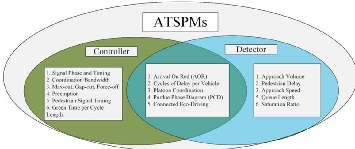
Figure 48. ATSPM Data Source and Performance Measurements
