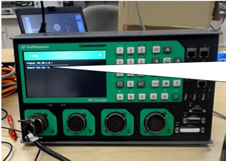
The PING will give a 'success' or 'timeout' type of response. If no RSU is setup, a 'timeout' should be received.
