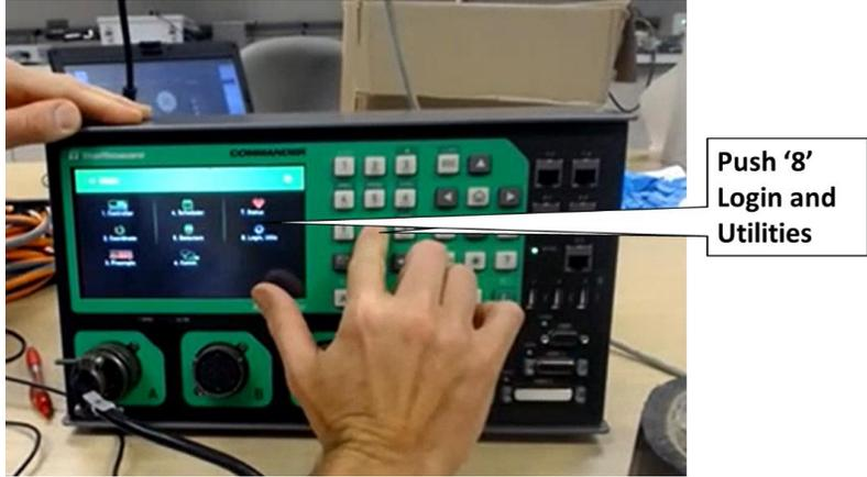
Figure 89. Trafficware Commander Initializing Controller-Utilities
