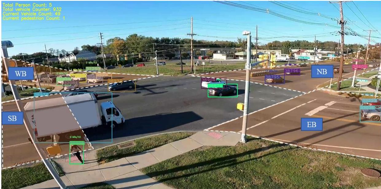
Figure 127. Sample of Road Users Detection Results
