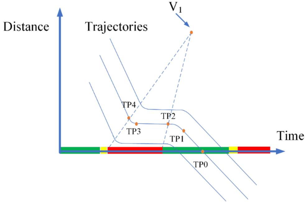
Figure 36. Under-Saturated: Turning Points used for Trajectory Reconstruction
