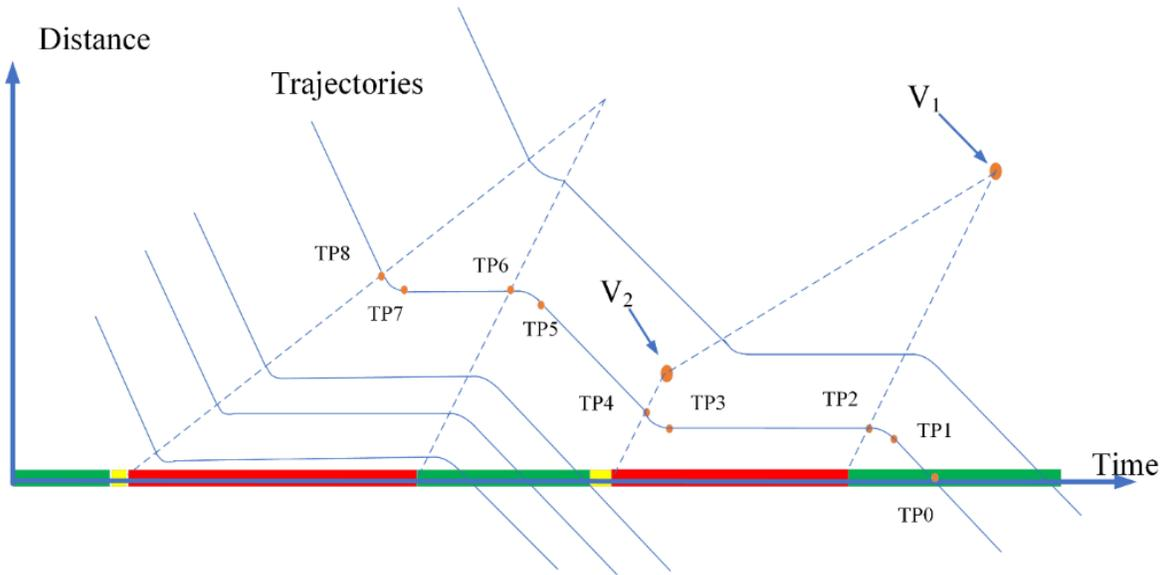
Figure 37. Saturated: Turning Points used for Trajectory Reconstruction
