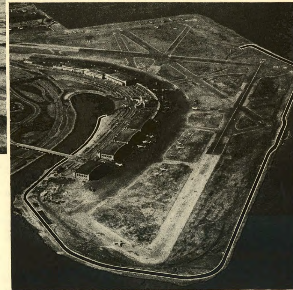
ABOVE: Flood waters lapping the La Guardia loading apron on October 30, 1947, before the construction of marginal dike. At right: Outline of the new marginal dike encircling the eastern half of La Guardia Airport.
