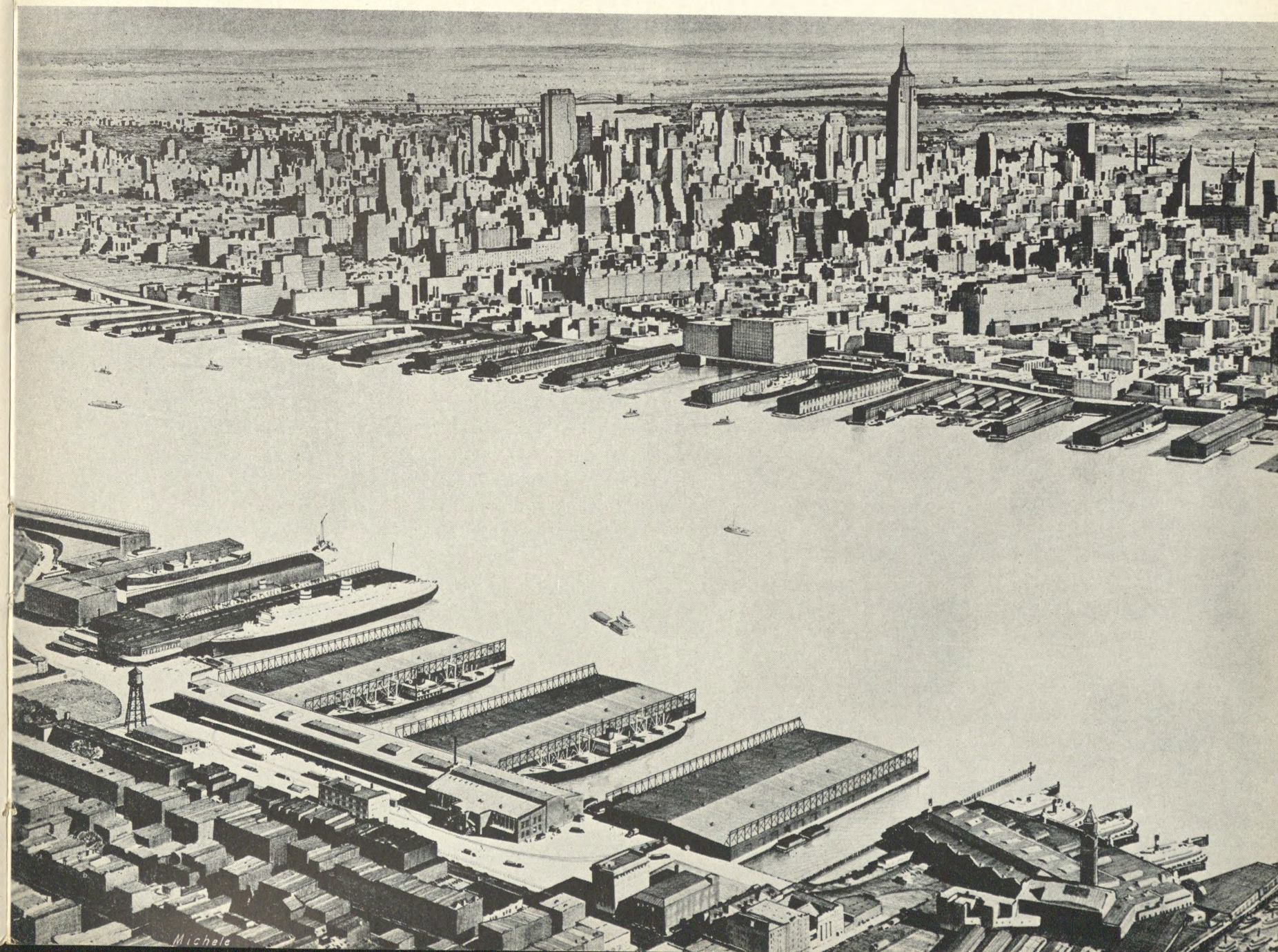
Artist's conception of proposed $22,000,000 Hoboken Pier development. Port Authority plan includes three-stage replacement of obsolete piers by one-story, steel and concrete fire-proof piers able to handle a million long tons of freight, double the present capacity.
