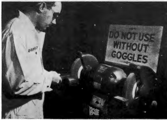
An example of a well-designed guard for a bench grinder. Note the side member of the guard is readily removed for access to wheel.
