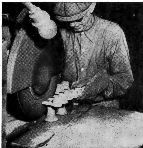
Cutting-off machine used to cut-off gates and risers. Note excellent guarding.
