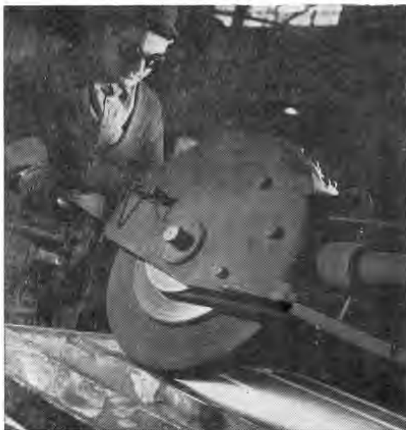
This swing frame grinder has an excellent guard. Note that the guard encloses at least 180° of the wheel.
