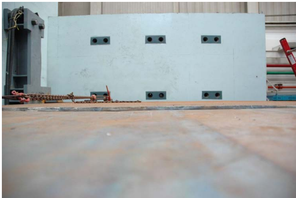
Figure 347. Elevation difference at splice location before tacking
