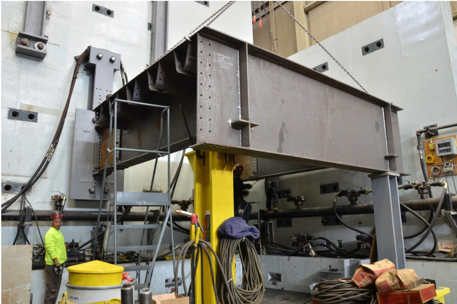
Figure 344. Installation of the east panel
