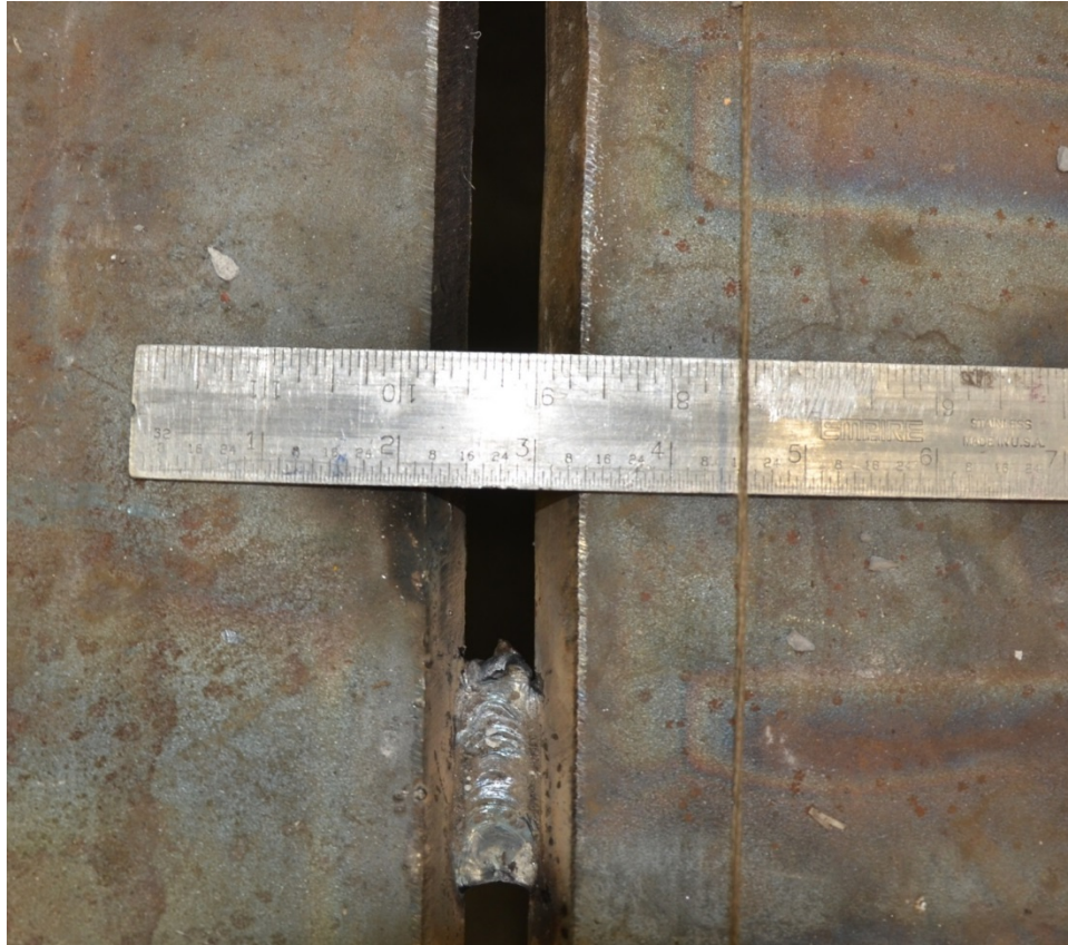
Figure 350. Maximum root gap of ½ in.
