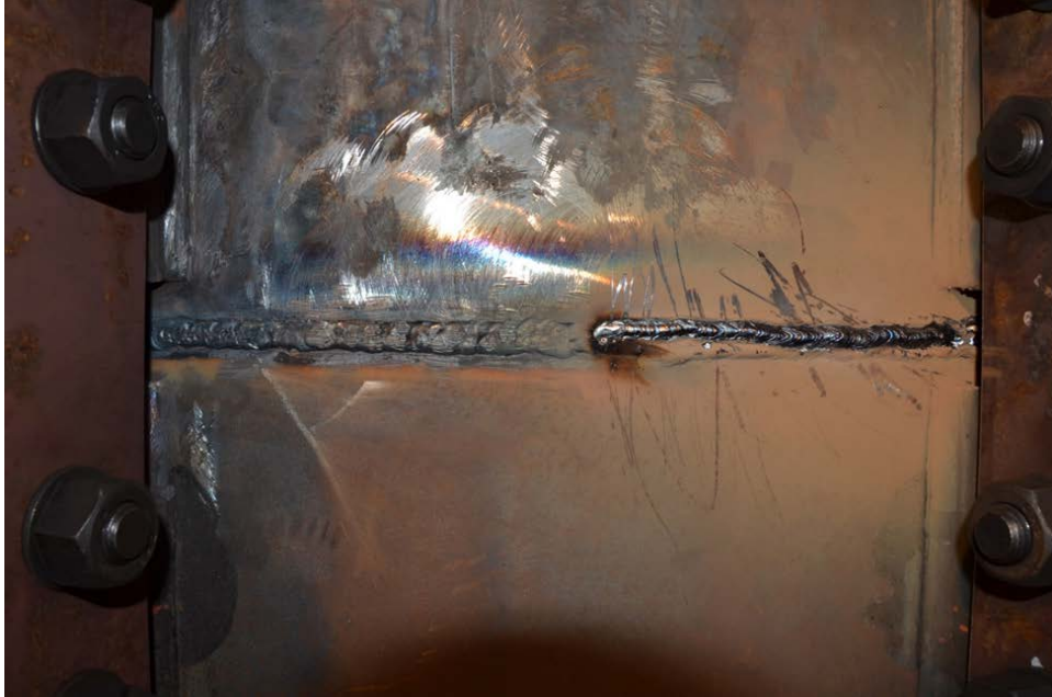
Figure 358. Weld root after re-welding
