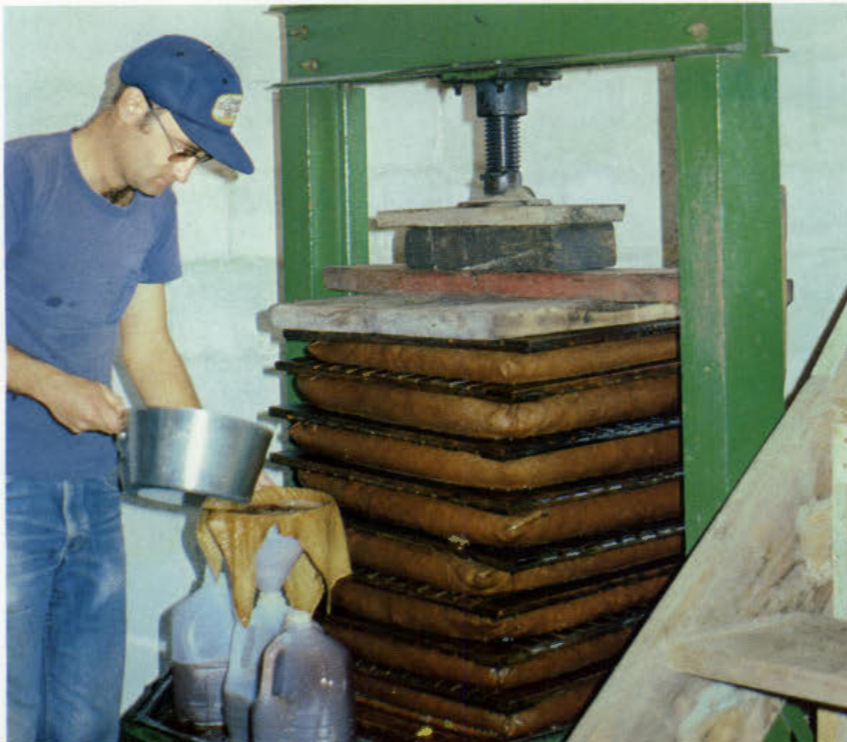
The cider is filtered through a double cheesecloth and bottled in gallon jugs. This New Jersey cider mill dates back to before Prohibition.
