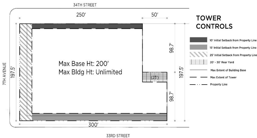
Figure IV-6.2 SITE 6 Tower Controls
