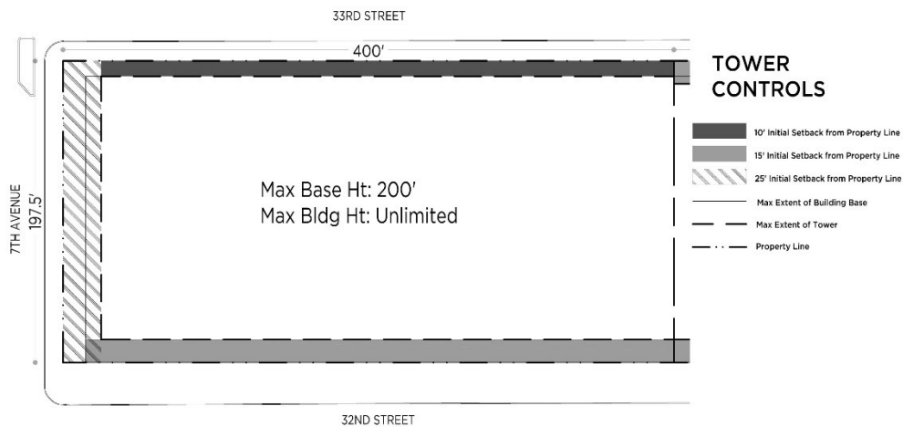
Figure IV-7.2 SITE 7 Tower Controls
