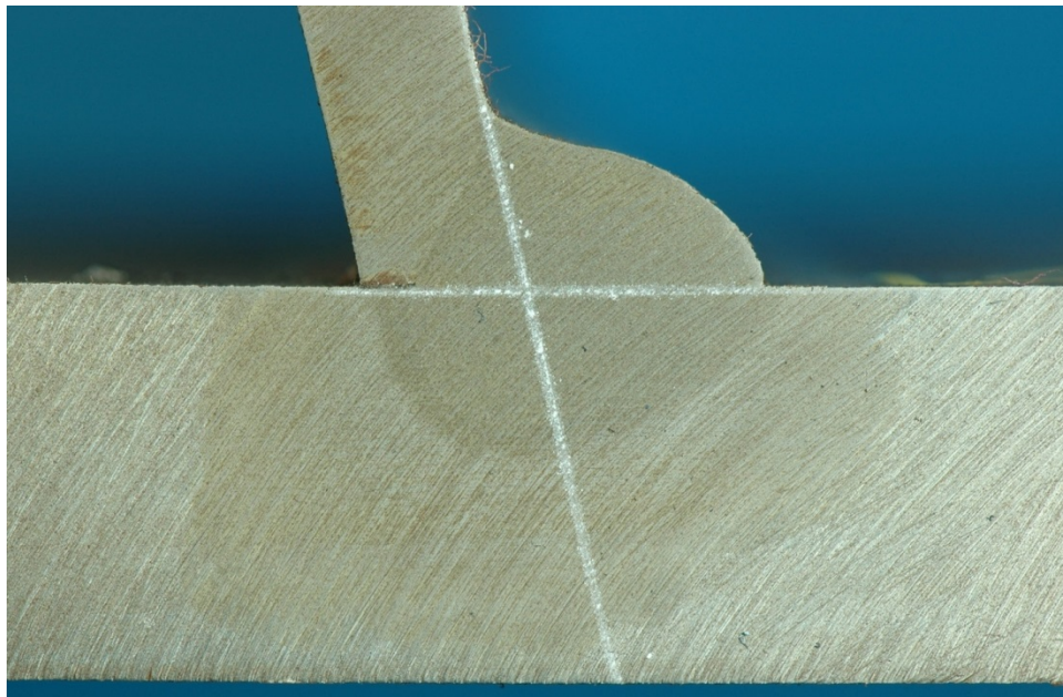
Figure 288. A typical macro-etched section for MU4
