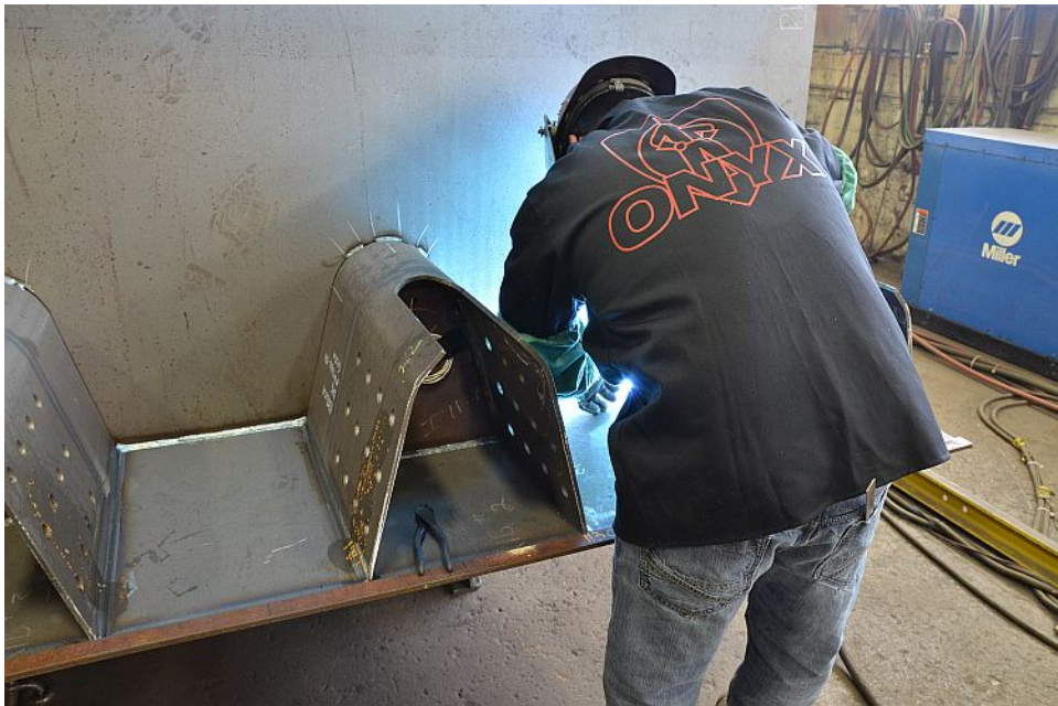
Figure 332. Floor beam-to-deck plate welding
