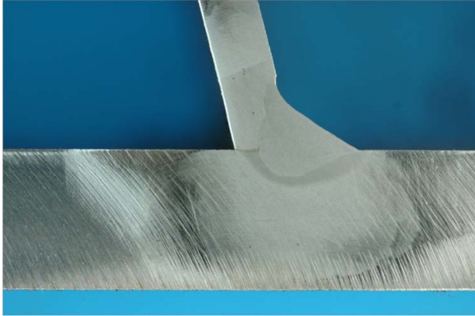
Figure 305. A typical macro-etched section for Rib 3 in MU5
