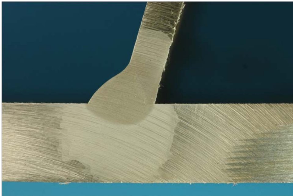
Figure 314. A typical macro-etched section for MU8
