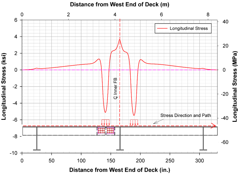
Figure 263. Variation of longitudinal stress on the top of the deck plate along a path through the south load pads
