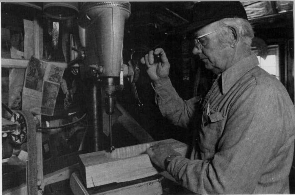
A modern drill press speeds the hollowing out of the inside of the decoy.
