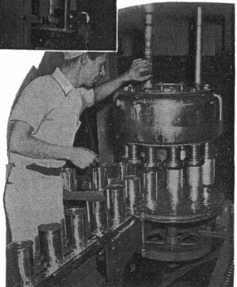
Cans being filled with tomato juice, and sealed, at a New Jersey processing house
