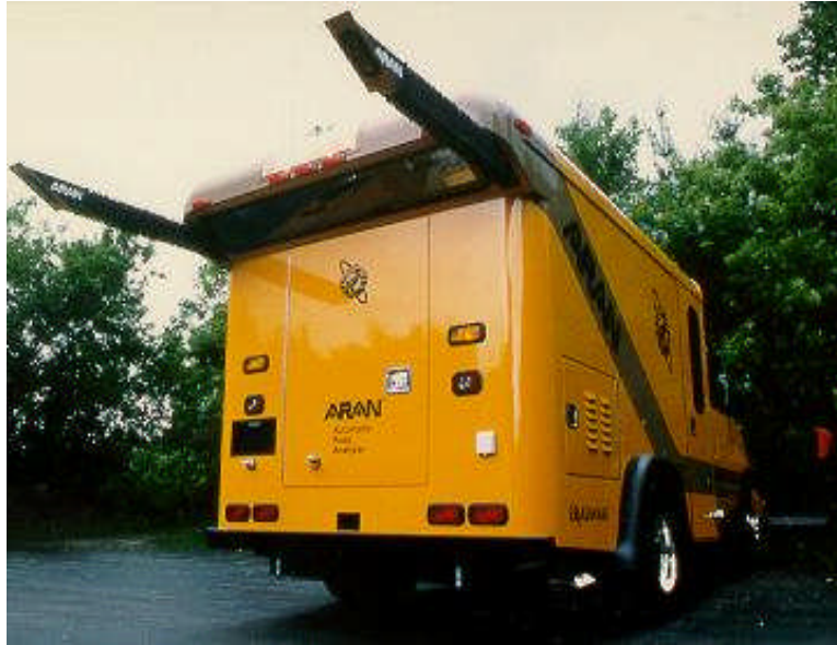
Figure 4. ARAN Dual Camera System
