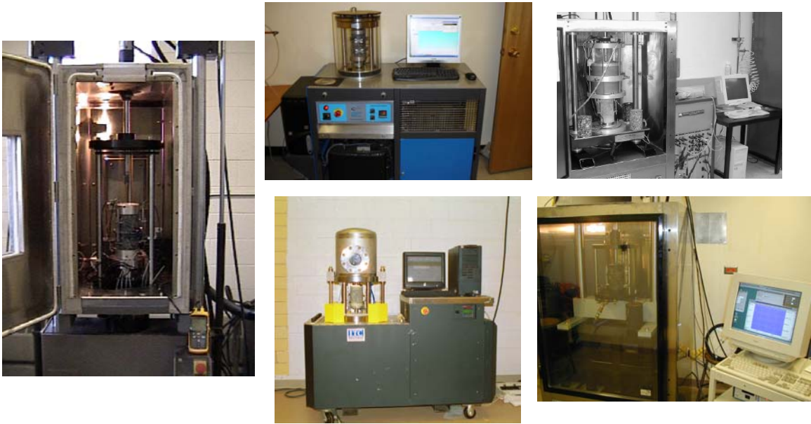
Figure 1 – Different Testing Machines Used to Measure the Dynamic Modulus of Hot Mix Asphalt
