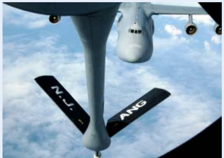
A C-5A Galaxy approaches the boom on one of the 108th Air Refueling Wing's KC-135E Stratotankers.
