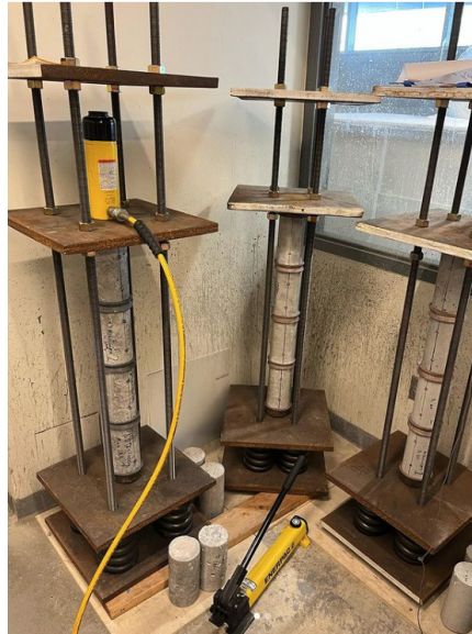
Figure 2. Creep frame with specimens under load
