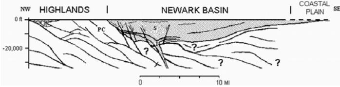
Figure 3. Schematic cross section showing crustal structure in the vicinity of the Newark Basin. The Newark Basin is filled with about 20,000 feet of Lower Mesozoic sedimentary (S) and igneous (I) rocks. Approximate section location shown in Figure 2 (CS). (PC -- Precambrian rock, S -- Paleozoic carbonate rock)
