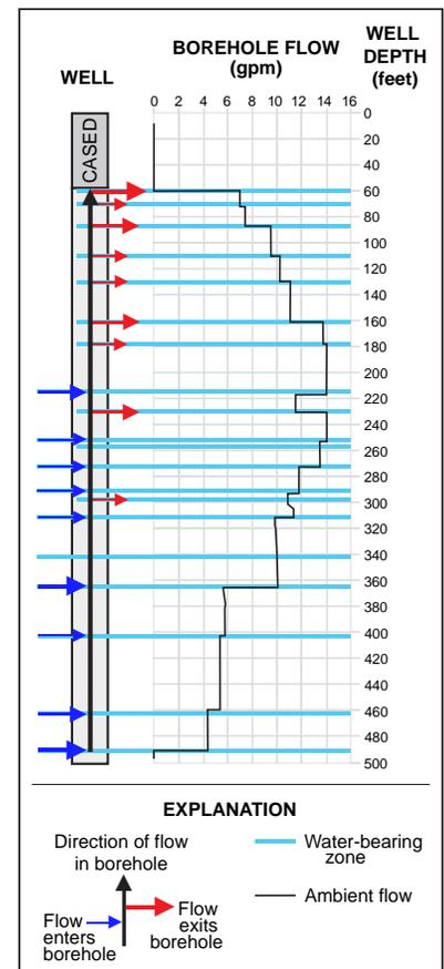
Figure 3. Diagram of borehole flow in OW-3. Data from G. Herman
