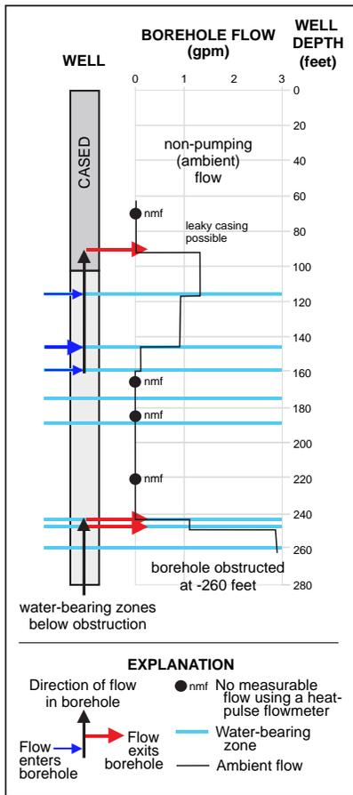
Figure 6. Diagram of borehole flow OW-2. Data from G. Herman
