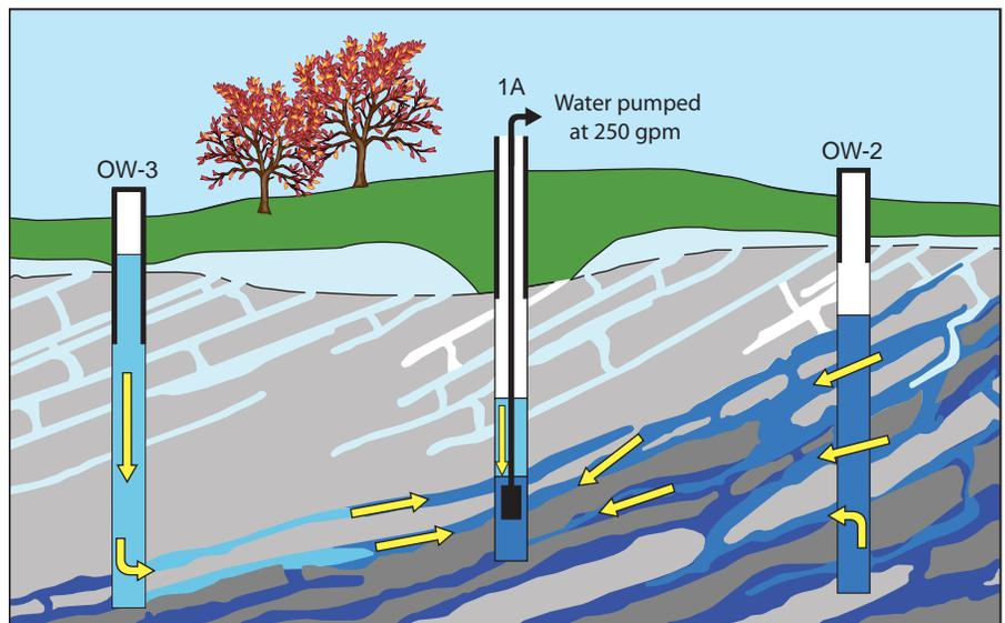
Figure 5. Schematic diagram of ground-water flow during pumping.
