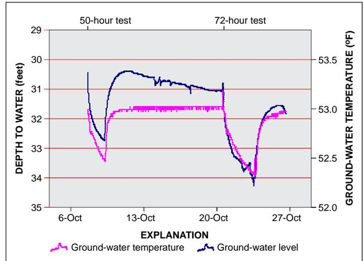
Figure 2. Hydrograph of OW-3 during aquifer tests.
