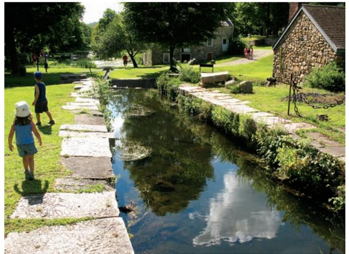
and also stored water to power the mill during dry periods. A raceway usually consisted of two parts, the head race (from the stream or pond to the water wheel) and a tail race (from the water wheel back to the stream). The height from which the water would fall when it reached the mill is called the head and determines the amount of water power. A shaft attached to the water wheel transmitted the power to the mill.
