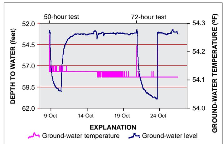
Figure 7. Hydrograph of OW-2 during aquifer tests.
