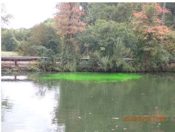
Dye testing for leaks being performed in canal above the Six Mile Run Culvert.
