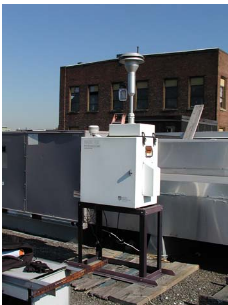
USEPA-approved manual PM 2.5 sampler on the roof of the Union City Health Department building in Hudson County
