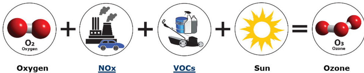
Figure 5.2. How Ozone is Formed. Ground-level ozone is formed when oxides of nitrogen (NO x ) and volatile organic compounds (VOCs) react in the presence of sunlight (NJDEP 2022a).
