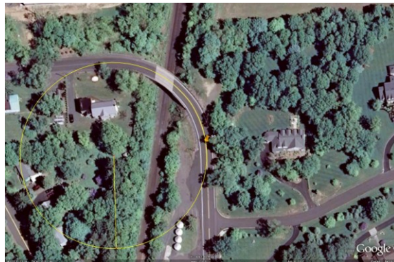
Figure 41. Example radius of curvature measurement from Google Earth Pro. This collision occurred in Mercer County on Route 640. The radius of curvature is 200 feet.
