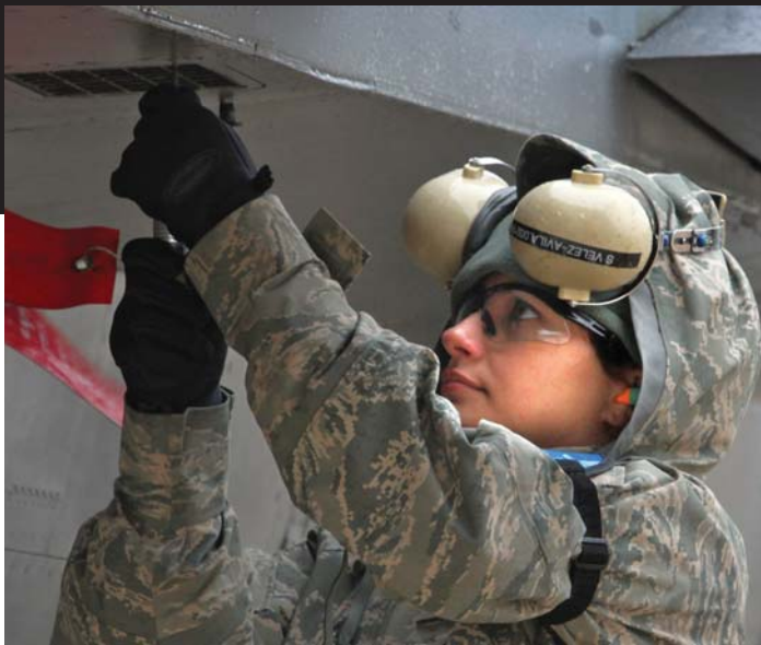
Left: Weapons Loader Staff Sgt. Sheila Velez-Avila installs a Chaff Module used to counter act radar guided missiles. Below: Lt. Col. Neal A. Snetsky flashes the Devil sign after landing his F-16 Fighting Falcon at "Base X".
