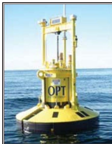
Ocean Power Technologies has successfully operated an autonomous PowerBuoy® off New Jersey, which it designed and manufactured under the US Navy's Littoral Expeditionary Autonomous PowerBuoy (LEAP) program for coastal security and maritime surveillance
