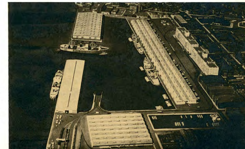
A close-up of reconstructed Atlantic Basin in southern area of Brooklyn-Port Authority Piers shows modern quays and warehouses. Seven ship berths will be provided in this area, including three at Pier 11 on the Basin's eastern side. This pier will be the first built under the Port Authority's development program.
