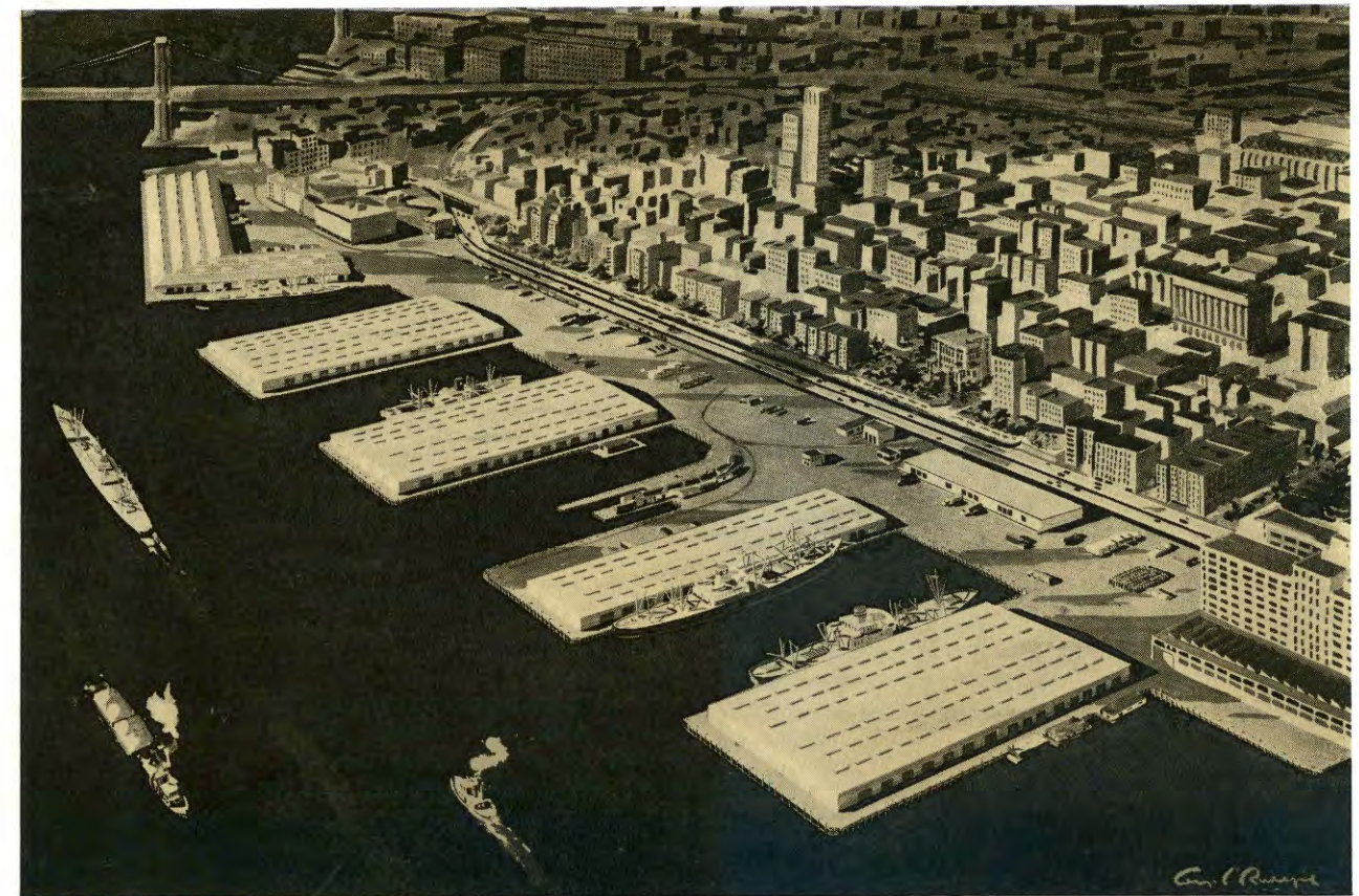
This artist's rendering shows the northern half of the Brooklyn-Port Authority Piers when modern steel and concrete structures will have replaced outmoded piers. Pier 1, the L-shaped structure immediately south of the Brooklyn Bridge, will provide two berths along its river frontage and a third berth on its south side.
