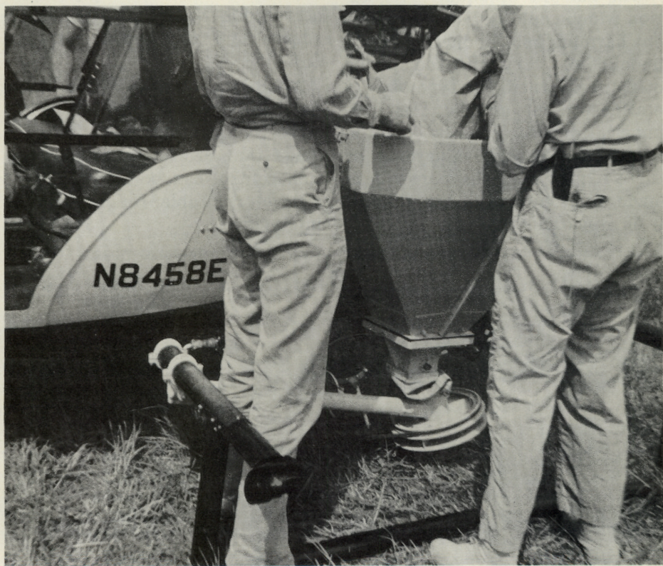
Loading granular herbicide into hopper mounted on helicopter
