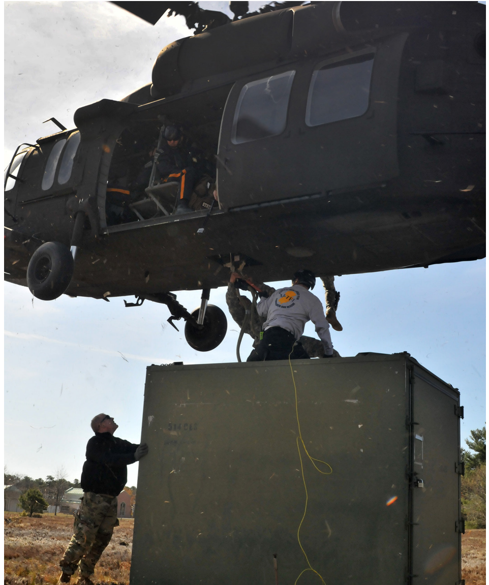
Members of 1-150th Assault Helicopter Battalion, Jersey Army Army National Guard, and the New Jersey State Police connect a sling loaded search and rescue gear container to a Black Hawk helicopter as part of a New Jersey Task Force 1 exercise.
