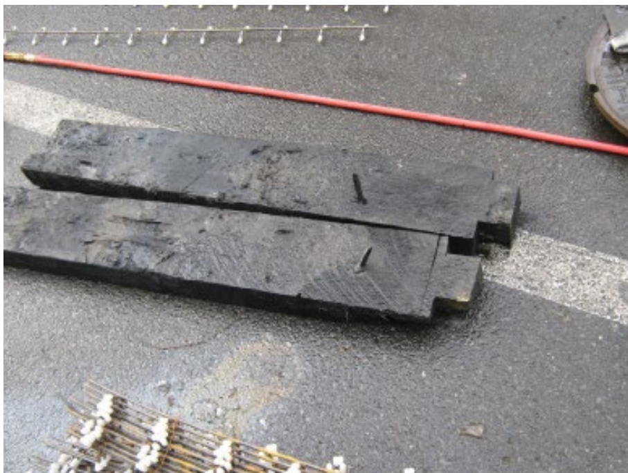
Figure 65. Metal spikes used in the construction of the Grand Street wood sewer, though notched ends were more common.
