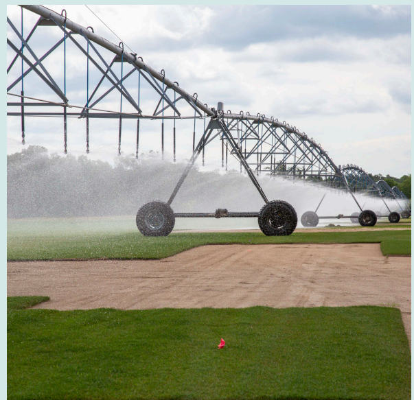
An overhead agricultural irrigation system at Tuckahoe Turf Farms in Hammonton, New Jersey. Climate change may increase water demands for agricultural irrigation by extending growing seasons and increasing the frequency of dry periods during the growing season.
