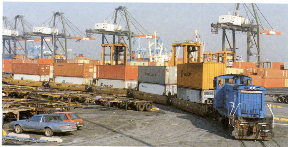
Conrail's new on-dock rail service at the Elizabeth-Port Authority Marine Terminal features double-stack trains—the most cost effective method of moving cargo by rail.
