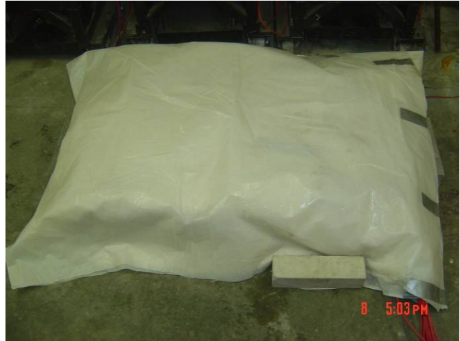
Figure 7. All Specimens Under Burlap and Polyethylene Sheet
