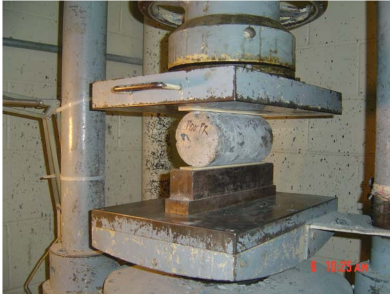
Figure 10. Splitting Tensile Strength Test Setup
