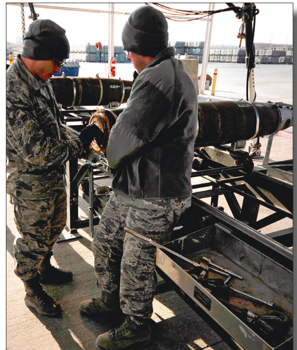
Photo top left, Airmen 1st Class Joe LaGreca, left, and Braun Hurley, right, detach the tail of a bomb undergoing a semi-annual compliance inspection at Bagram Airfield. Photo top right, LaGreca inspects the components of an MK82 bomb body during an assembled munitions serviceability inspection. LaGreca is a Guardsman from the 177th Fighter Wing, Atlantic City. (U.S. Air Force photos by Tech. Sgt. Vernon Cunningham, 455th AEW/PA)
