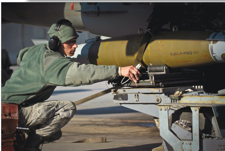
Photo top left, Airmen 1st Class Joe LaGreca, left, and Braun Hurley, right, detach the tail of a bomb undergoing a semi-annual compliance inspection at Bagram Airfield. Photo top right, LaGreca inspects the components of an MK82 bomb body during an assembled munitions serviceability inspection. LaGreca is a Guardsman from the 177th Fighter Wing, Atlantic City. (U.S. Air Force photos by Tech. Sgt. Vernon Cunningham, 455th AEW/PA)
