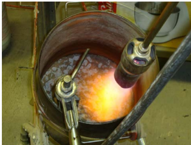
Figure 15. Heating and Mixing Aggregate Blend
