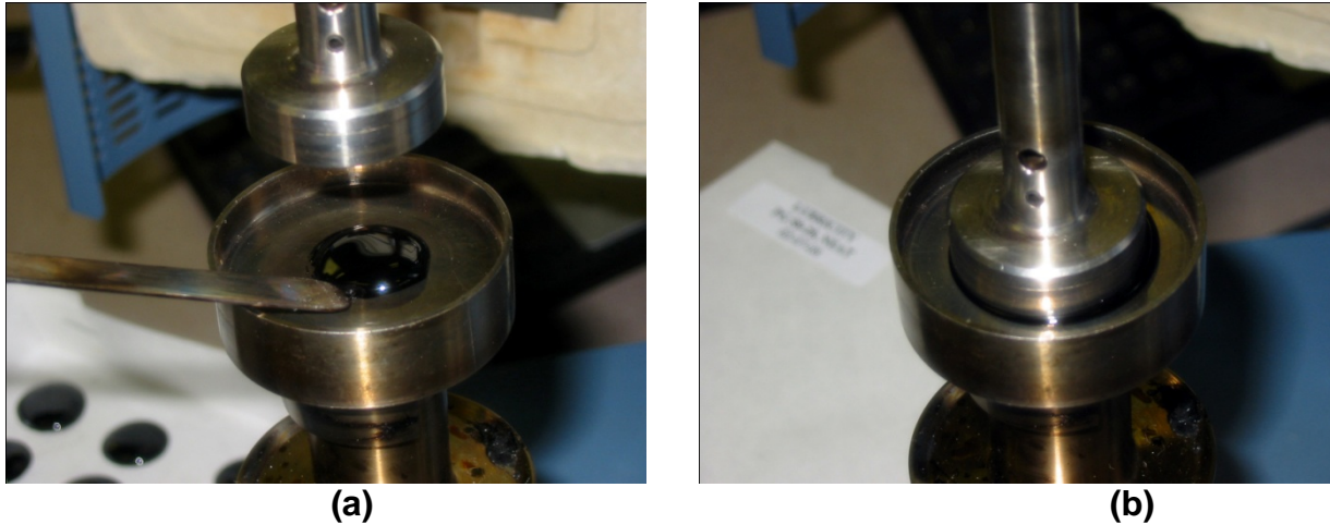
Figure 18. Lubricity Test Setup a) Loading Asphalt Binder Pat in Bottom Cup Platen; b) Lowering Top Platen to 100 Microns
