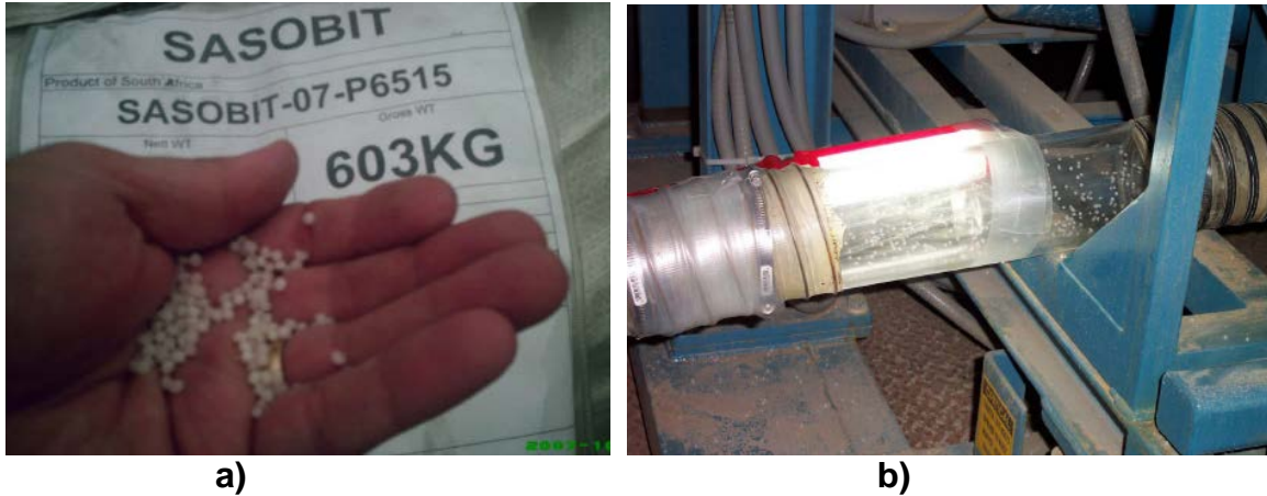
Figure 5 – a) Sasobit Pellets and b) Sasobit Being Blown into Drum Plant
