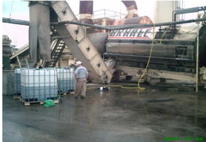
Figure 2. Evotherm Added to Drum (85% Water; 15% “Chemical Package”)
