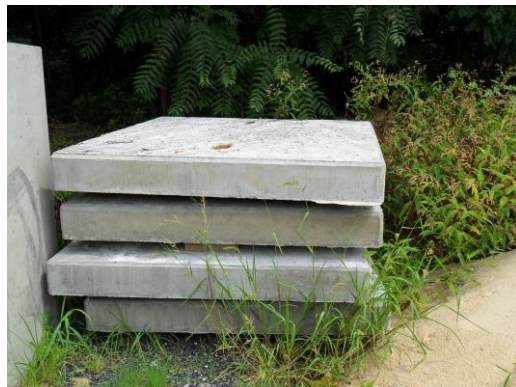
Figure 12. Items precast using recycled concrete aggregates
