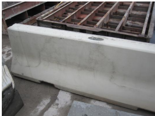
Figure 12. Items precast using recycled concrete aggregates
