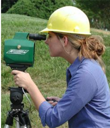
Figure 43. A laser based system to measure distances and angles
