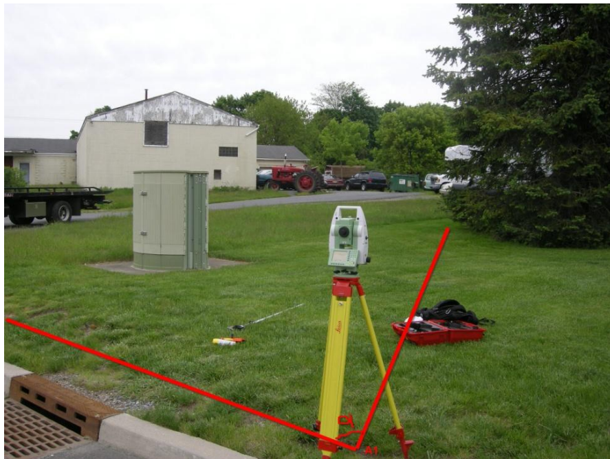
Figure 50. Use the laser system to find the predetermined sight angle \alpha
