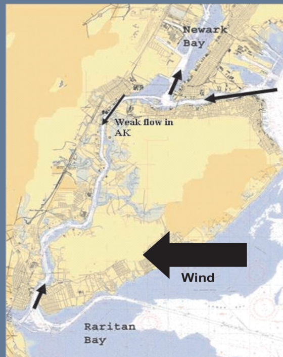
Figure 9: Tidal Residual Currents during Strong, Large-Scale Winds from the West (left panel) and the East (right panel).
