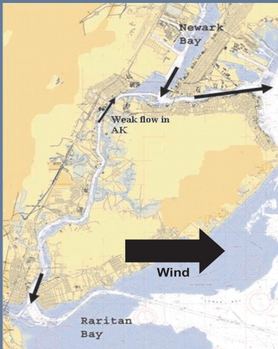
Figure 9: Tidal Residual Currents during Strong, Large-Scale Winds from the West (left panel) and the East (right panel).
