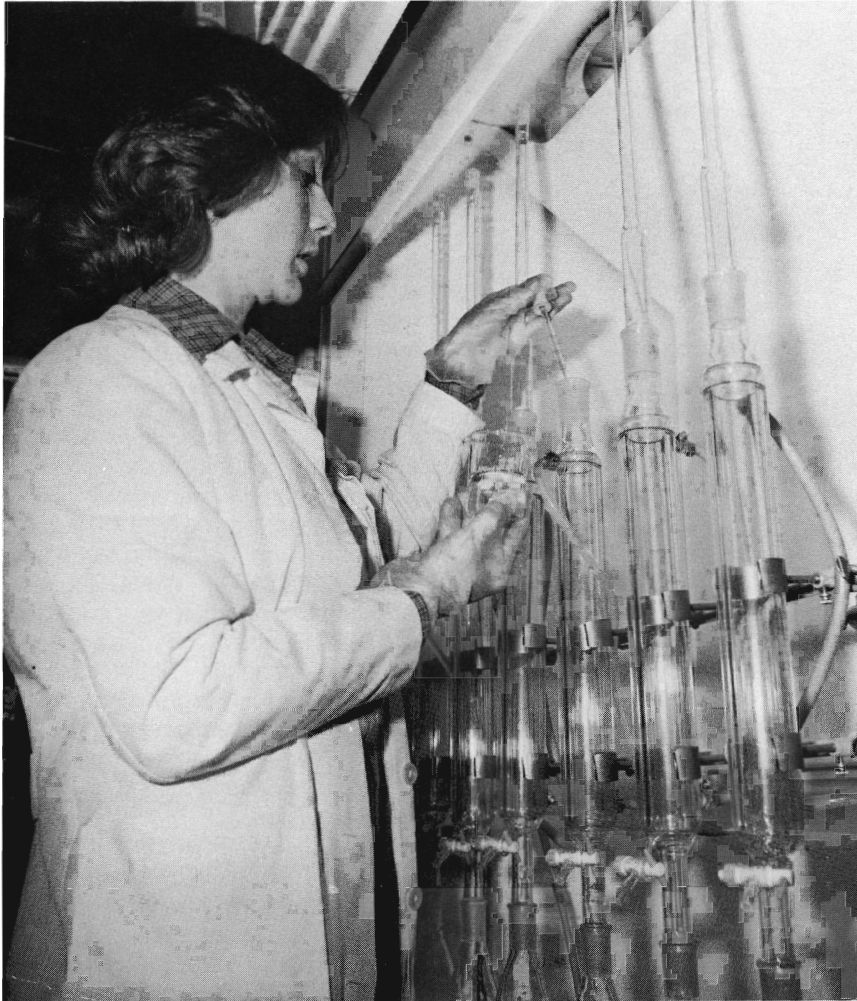
Researcher applies a water sample to an extraction column in order to identify the type of chemicals in the sample.
