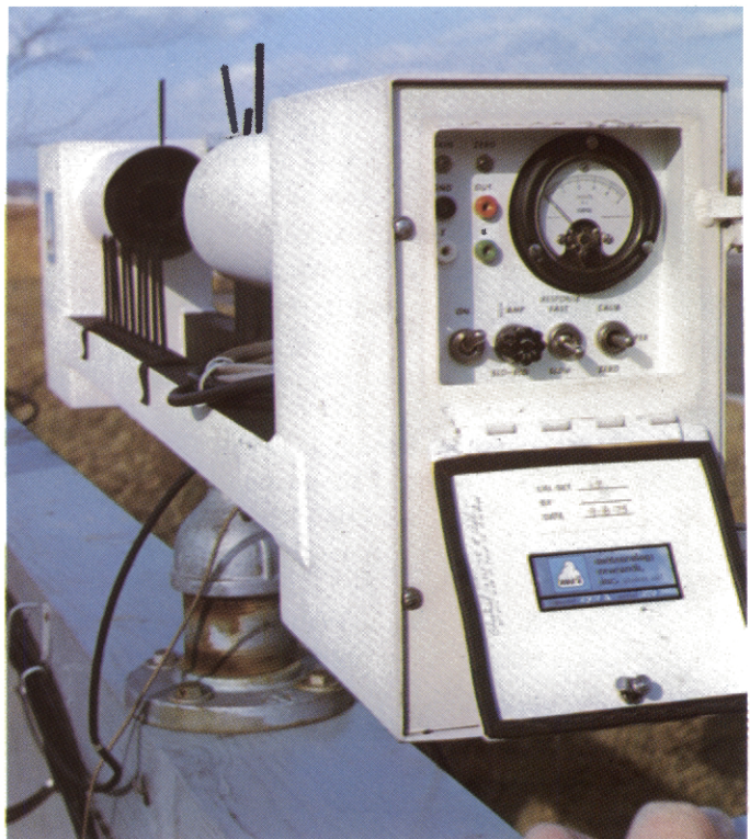
One of the five fog detectors being tested at Interchange 16W in fog-prone meadowland area.
