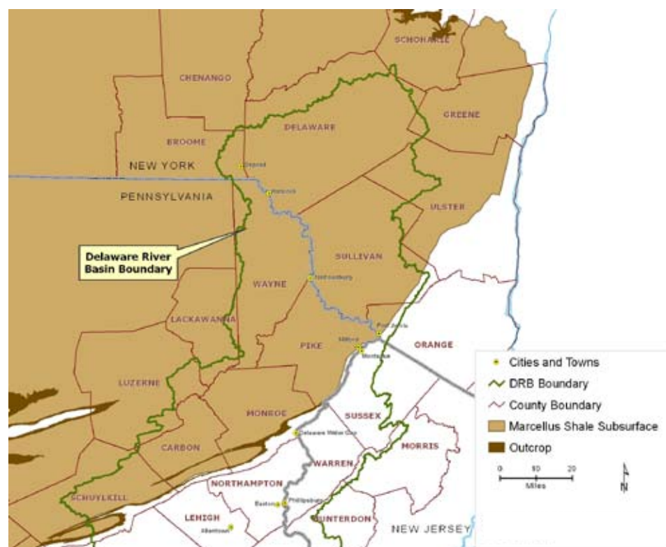
This map shows the extent of the Marcellus Shale formation in the Delaware River Basin (DRB). “Outcrop” refers to shale formations found at surface level. (Source: USGS National Assessment of Oil and Gas)
