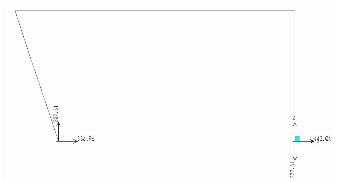
Figure VII.A.56 Pier 3 Transverse Reactions Lateral 2
