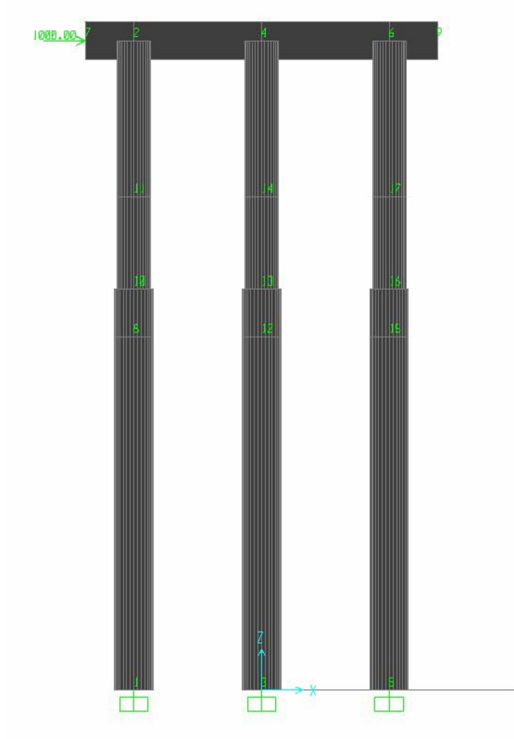
Figure VI.A.36 CSI-SAP Model 4 Subjected to 1000 Kips of Transverse Loading
